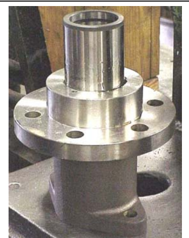
Figure 12, RBS bushing installation
