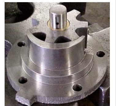
Figure 5, Pressing the idler pin
