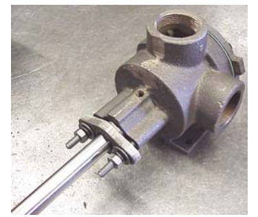
Figure 11, Gland & fasteners installed
