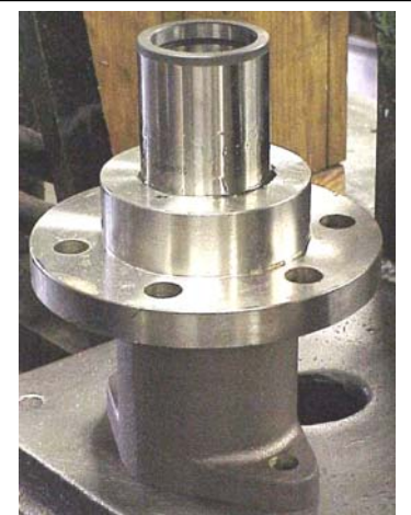
Figure 12, RBS bushing installation
